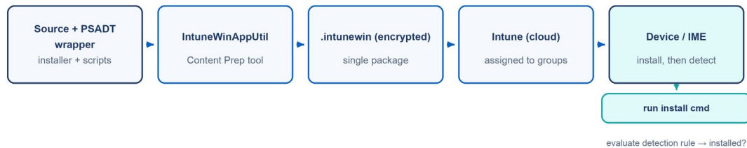
Figure 10.2: The Win32 packaging pipeline — source plus a PSADT wrapper is compiled by IntuneWinAppUtil into an encrypted .intunewin, uploaded to Intune, and pulled down by the Intune Management Extension, which runs the install command and then evaluates the detection rule to decide whether the app is present.
